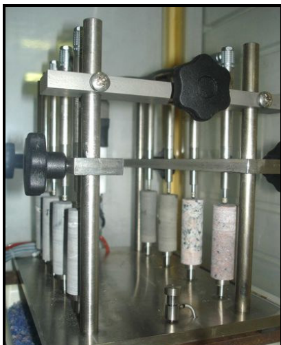
Figure WP3.1 - Hygric and thermal dilatometric system developed during the project.
