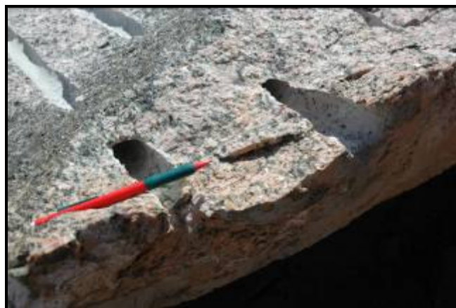
Figure WP2.1 - Different alteration patterns affecting the surface of a modern granite block in the South Mahmoudia quarry: - the scaling pattern is visible on the surface of the block - inter and intra granular cracks affect the block mainly in its subsurface - the iron oxide content coming from the alteration of ferromagnesian primary minerals seems to decrease from the surface to depth
