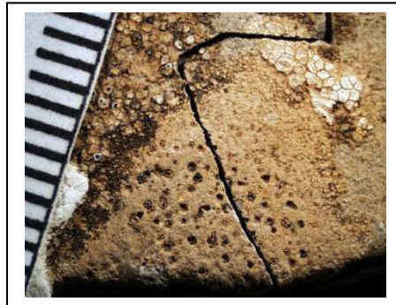
Figure WP2.6 - Pitting occurring on the surface of a limestone due to the endolithic lichen growth
